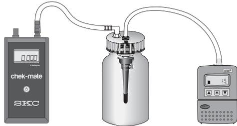
*Figure 3. Calibration Train with Jar*
